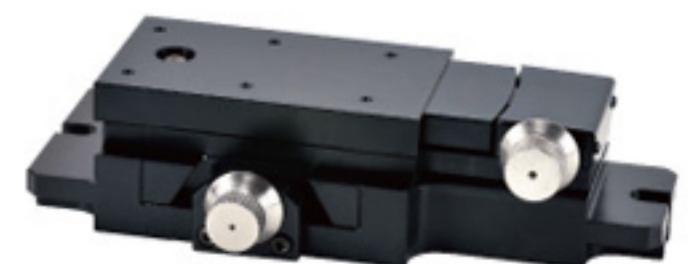
Model No.: AF-282 • Micro cross-travel table (Yθ) • Dovetail type • Dimension : 260 x 100 x 62mm • Yθ travel : ±12.5mm, θangle±5
